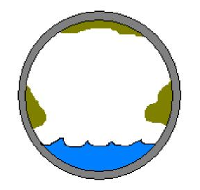
The start of a blocked pipe begins when grease collects on the top and sides of the pipe interior.
