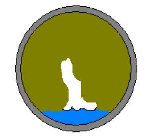
Excessive accumulation will restrict the flow of wastewater and can result in a sanitary sewer overflow.
