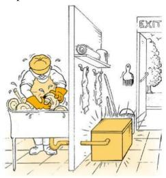
**Grease traps:** These are small devices connected directly to the outgoing drains of sinks inside the restaurant. Grease traps are designed to retain FOG usually from one fixture. Because they hold small quantities of captured FOG, such traps must be cleaned frequently (e.g. daily, weekly).
